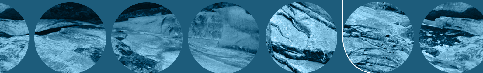
Figure 4: T 1 -T 2 maps of shale at various temperatures.
